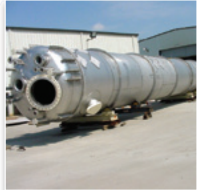
Duplex reactor fabrication for shipment and installation
