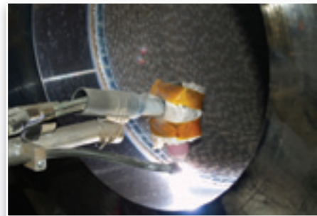
Automated manipulator overlaying nickel alloy
