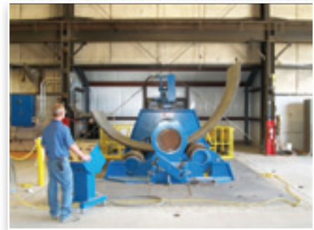
Plate roll forms up to 3.5" thick plate, 10' wide
