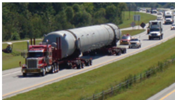
Oversize shipment of 140 ton, 180-foot long, 2-inch shell thickness distillation column with internal attachments.
