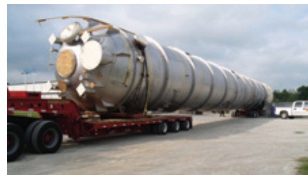
Oversize shipment of a reactor vessel made with Duplex 2205 alloy material.
